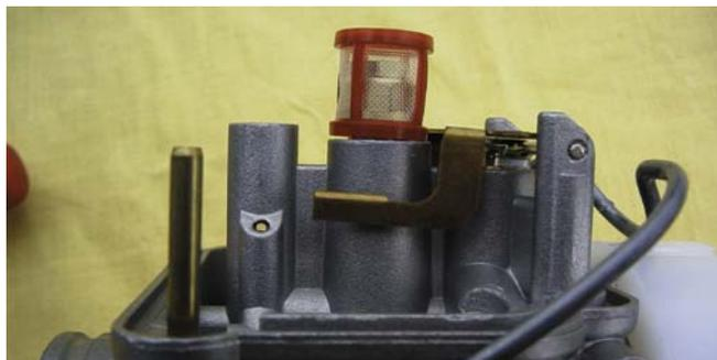
Before you start the cold motor press down the choke. Start the motor and after a few seconds release the choke.
