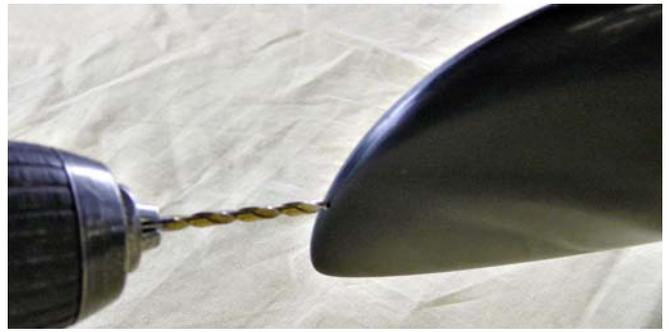
**Attention:** An imbalanced propeller created unnecessary vibration in the engine and can destroy many of its components.
