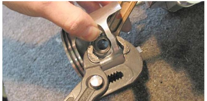
To the piston belongs two different rings. The upper ring is marked with a "0". This is faced to the top.
