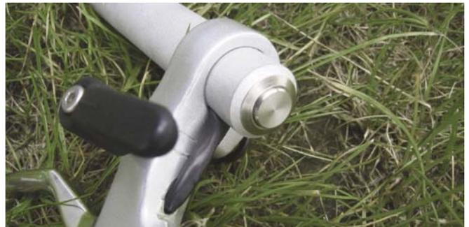
The throttle has also a travelling locking. After reaching the desired height of flight, the throttle can be fixed via the clasp-lever. Since long holt of the throttle is hard in hand, the throttle can be placed in position onto the legs. The hand are now free for other things.
