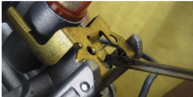
If you hold the carb up side down, the swimmer for is not parallel to the carburettor case. If the carb overfloat while using the motor the for should look a little bit more upward.
