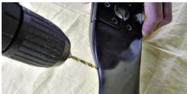
Then fill only as much resign into this hole until the propeller does not want to turn to one side only.
