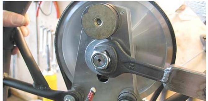
2. Lift the rotor-hub with the tension-screw (5mm) in order for the belt to either tighten or subside, thus the belt can be loosend. Turn right-belt tighten. Turn left-belt loosens.
