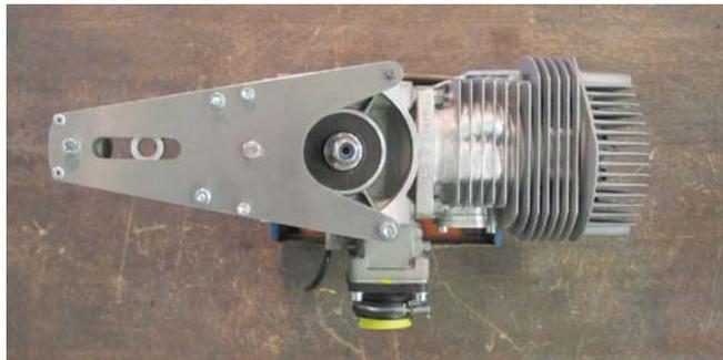
In flight the motor will become very hot. The most stressed area are the piston and the rings. Remove the exhaust and have a look to appeared piston with it's rings. Test it with screwdriver. The rings should be loose inside the slot.
