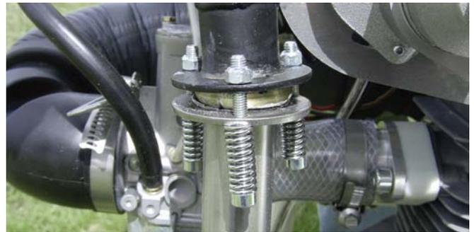
After 10 hrs the sealing-rings and their fasten screws needs to be checked. The screw you have to changes each 25 hrs.
