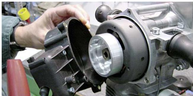
Once the central screw has been removed, the rotor can then be pulled off via a puller. Because the rotor has to be in a specific position to the crankshaft, the rotor with a suspension-disc on the crankshaft is preordained.
