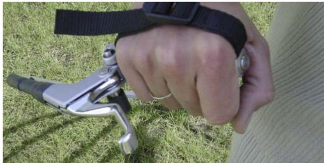
The Respect-throttle-lever has in each case a switch at the tube. The one is for the starting the engine.
