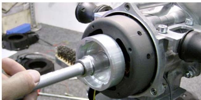
To fine-tune the ignition timingpoint one has to loosen the two security screws of the stator. Turn the stator to the left maximally to the furthest point, now turn ca 2 mm to the right again. Retighten the security screws. The ignition timingpoint has now its correct adjustment. When reassembling take special care of the correct distance of the contact-test that the distance of 0,25 mm is observed and if necessary readjust.
