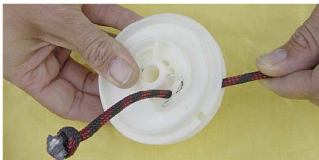
To give the starter-rope advanced tension one,place the rolled up into the slot and rotate three times.
