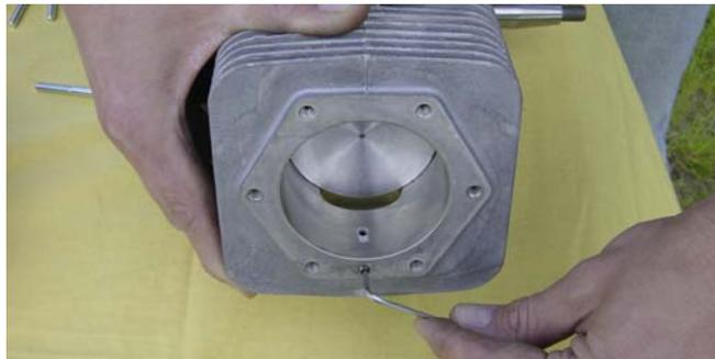
To reopening the hole use a 3,5 mm drill. Bore from top and from inside the cylinderwall with an angle from 45°.
