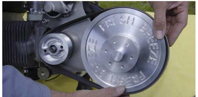
If the belt makes squeaking noises in spite of the proper tension, then spray twice onto the lower pulley. If the belt is slipping in spite of proper tension, then it needs to be replaced.
