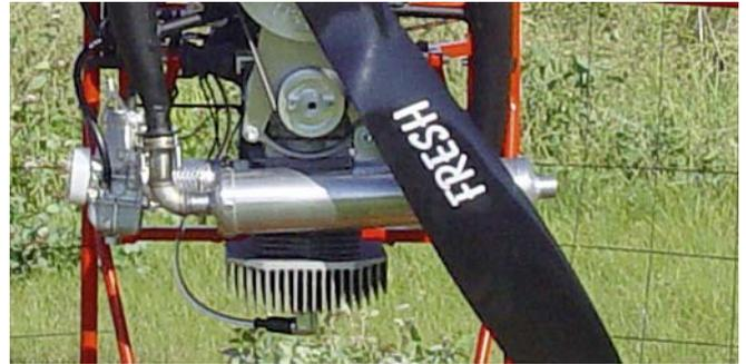
To keep the exhaust flexibly mobile we chose different types of fixtures. One is a rubber connection on the gear-plate and two a stress-bearing spring-gasket at the entry and the exit.
