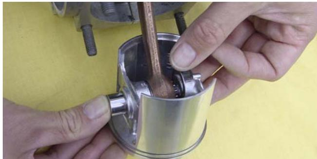
This picture demonstrate the spezial tool how to remove the safety ring.
